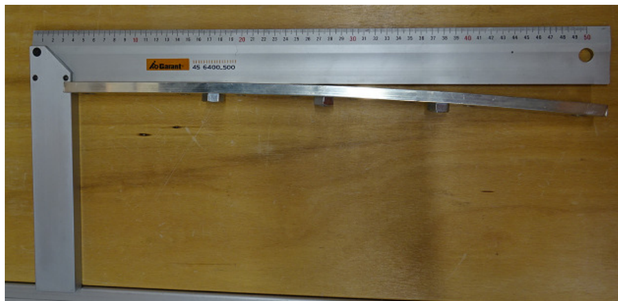
figure 13: Busbars not straight
